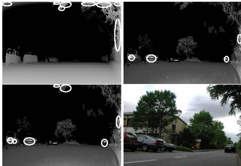
Fig. 6.11. The foci in laser data show some advantages of the reflection mode. In reading order: depth image, reflection image, combined image, camera image. All of the four cars are among the first six focus regions in the reflection data
