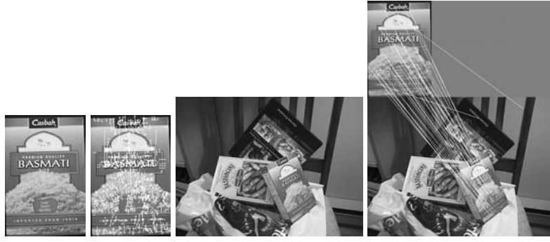
Fig. 7.7. Testing Lowe's SIFT Keypoint Detector [Lowe, 2004, URL, 13] for a complex target (basmati rice box). From left to right: 1) Training image. 2) 572 keypoints on training image. 3) Test image. 4) Test image in which 38 keypoints match. For such complex target objects, the recognition is successful even if the target is presented from different viewpoints (original images from [URL, 13])
